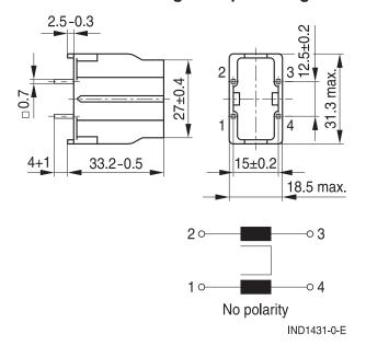
Part tolerances to ISO 2768-cL / ISO 8015. Size ISO 14405 (E) All dimensions in mm
