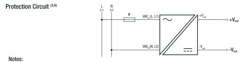
Note6: An external fuse is mandatory in order to protect the device in addition on the AC input side. RECOM recommend: slow blow type, 600Vac, 2A.
