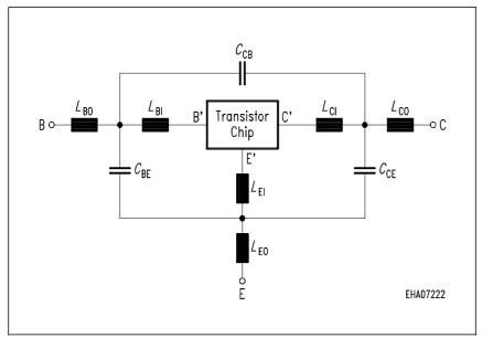
The TSFP-4 package has two emitter leads. To avoid high complexity fo the package equivalent circuit, both leads are combined in one electrical connection.
