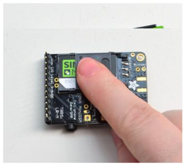
Close the hinge down and slide the cover to lock it in place
