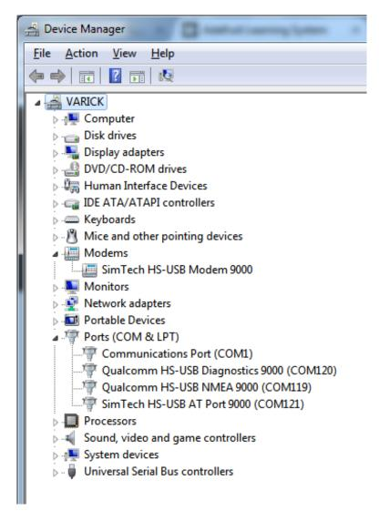
You can connect to the AT com port at any baud rate and send AT commands like normal. This makes it super easy to test out commands
