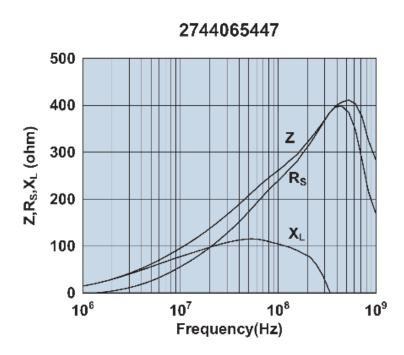
Impedance, reactance, and resistance vs. frequency.
