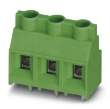
PCB terminal block, nominal current: 32 A, rated voltage: 690 V, pitch: 9.5 mm, no. of positions: 3, mounting: Soldering, type of connection: Screw connection, connection direction from the conductor to the PCB: 0°
