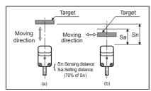
Sensing distance can be changed by the shape, size or material of the target.
