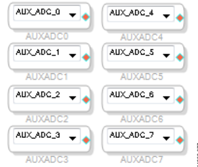
Figure 78. Complete Set of Auxiliary ADC Inputs in SigmaStudio
