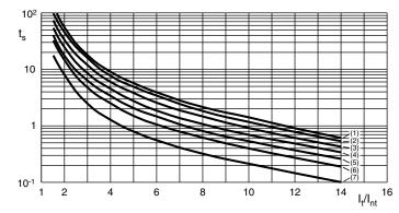
Curve 2:  $\varnothing$  D<sub>max.</sub> = 16.5 mm Curve 3:  $\varnothing$  D<sub>max.</sub> = 12.5 mm Curve 4:  $\varnothing$  D<sub>max.</sub> = 10.5 mm Curve 5:  $\varnothing$  D<sub>max.</sub> = 8.5 mm Curve 6:  $\varnothing$  D<sub>max.</sub> = 7.0 mm Curve 7:  $\varnothing$  D<sub>max.</sub> = 5.0 mm
