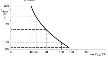
$I_{\text{max.}}$  as stated in the electrical data and ordering information tables, is the maximum overload current that may flow through the PTC when passing from the low ohmic to high ohmic state at rated voltage.
