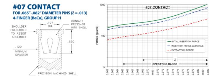
The insertion / extraction force characteristics above were derived using a 30 microinch gold-plated contact and polished steel gauge pins having a bullet-shaped tip.
