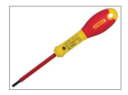
The Stanley FatMax Parallel Tip VDE Insulated Screwdrivers have a VDE insulated screwdriver tip that is individually tested to 10,000 volts and guaranteed to 1,000 volts. The soft-grip handle gives the perfect combination of great grip plus reduced fatigue and its large diameter offers greater torque needed for driving wood screws.
