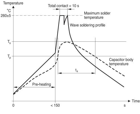
$T_s$ : Capacitor body maximum temperature at wave soldering  $T_p$ : Capacitor body maximum temperature at pre-heating  $\kappa$
