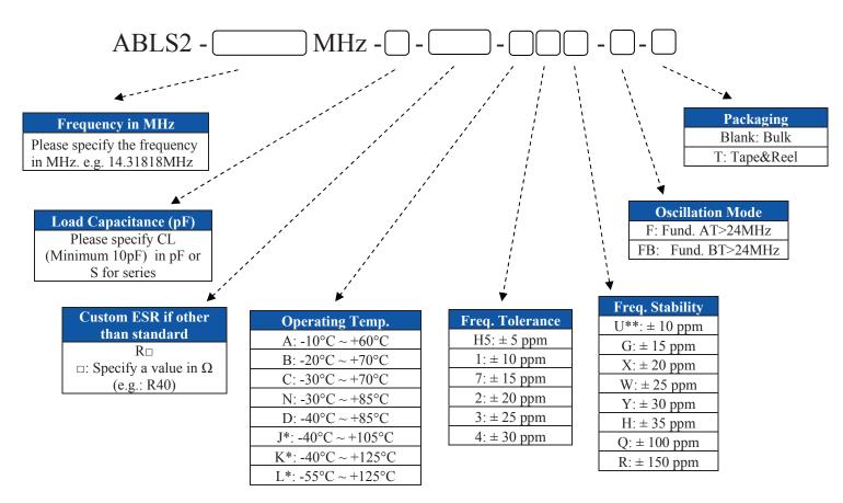
NOTE: Fundamental BT frequency stability  $\pm$  100ppm max. at -10° C to +60° C only.
