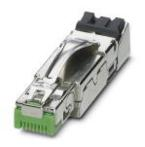
RJ45 connector, degree of protection: IP20, number of positions: 6, 100 Mbps, CAT5 (IEC 11801:2002), material: Zinc die-cast, connection method: IDC fast connection, connection cross section: AWG 26- 24, cable outlet: straight, High degree of resistance to vibration; 360° shielding; one-piece design; special tool-free assembly
