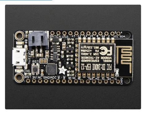
At the Feather HUZZAH's heart is an ESP8266 WiFi microcontroller clocked at 80 MHz and at 3.3V logic. This microcontroller contains a Tensilica chip core as well as a full WiFi stack. You can progam the microcontroller using the Arduino IDE for an easy-to-run Internet of Things core. We wired up a USB-Serial chip that can upload code at a blistering 921600 baud for fast development time. It also has auto-reset so no noodling with pins and reset button pressings.
