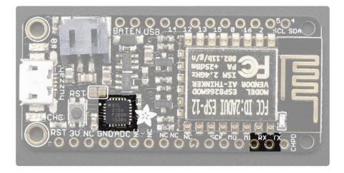
The TX pin is the output from the module and is 3.3V logic.
