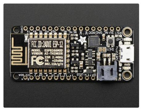
While the Feather HUZZAH ESP8266 comes pre-programmed with NodeMCU's Lua interpretter, you don't have to use it! Instead, you can use the Arduino IDE which may be more familar. This will write directly to the firmware, erasing the NodeMCU firmware, so if you want to go back to Lua, use the flasher to re-install it (https://adafru.it/fIO)
