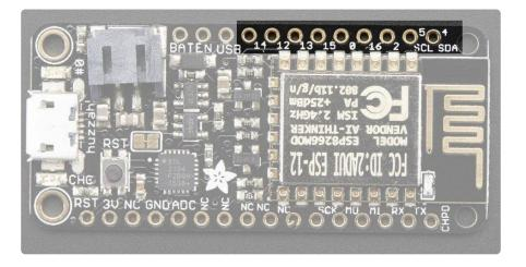
This breakout has 9 GPIO: #0, #2, #4, #5, #12, #13, #14, #15, #16 arranged at the top edge of the Feather PCB
