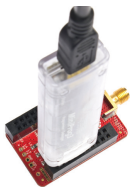
Fig-2: Programming and Debugging with CY8CKIT-002
