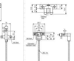
\*When using photoelectric sensors closely over two units, it may result in malfunction due to mutual interference. When installing the product, tighten the screw with a tightening torque of 0.49Nm •BS5-Y1M / BS5-Y1M-P M3 Bolt
