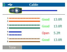
Cable test showing pairs 4 and 5 are open.
