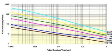
This data is for the  $100\Omega$  resistance value for each size. Pulse power handling is dependent on the resistance value. For resistance values higher or lower than  $100\Omega$ , contact Stackpole for advice on pulse handling characteristics of your particular resistance value of interest.
