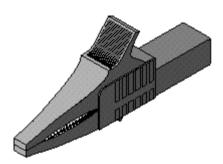
Fully insulated banana-jack alligator clips. Extra strong teeth and new spring design provide superior grip. Extremely rugged. Large .787" (20 mm) opening. 600V per IEC 1010, Overvoltage Category III (Heavy Industrial Rating), 10A rating. One red, one black.
