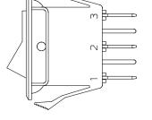
NOTE: Orientation of actuator marking and terminals.
