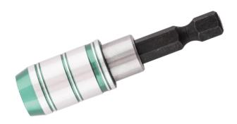
RS Pro Magnetic EasyLink/EasyLock bit holder is a quality bit holder packed with features. Inserting and removing the bit is possible with one hand operation. To insert and lock the bit in place, simply push the bit into the holder without actuating the functional sleeve. To unlock, actuate the functional sleeve and the bit is unlocked and pushed forward. Supplied in a compact plastic box.
