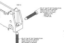
'anhead Thread Cutting Screw: 4-24 X 5/16" ype: USA Std BT, Federal BG
