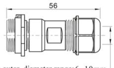
Cable outer diameter range: 6-10mm
