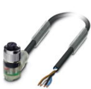
Sensor/Actuator cable, 4-position, PUR halogen-free, Black-gray RAL 7021, Free cable end, on Socket angled M12, A-coded, with 3 LEDs, Cable length: 10 m
