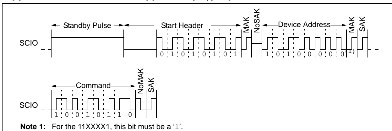
FIGURE 4-4: WRITE ENABLE COMMAND SEQUENCE
