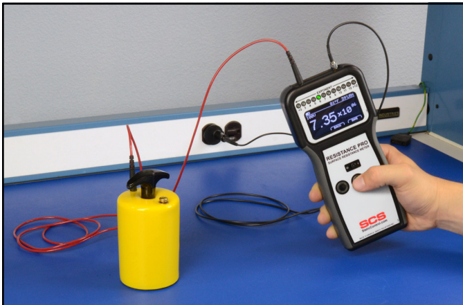
Figure 8. Measuring the Resistance-to-Ground (Rtg) of a worksurface mat
