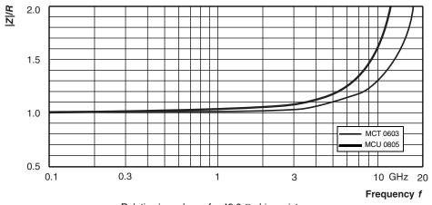
Relative impedance for 49.9  $\Omega$  chip resistor
