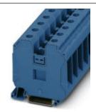
Feed-through terminal block, nom. voltage: 1000 V, nominal current: 125 A, connection method: Screw connection, number of connections: 2, cross section: 1.5 mm² - 50 mm², AWG: 16 - 1/0, width: 16 mm, height: 65.1 mm, color: blue, mounting type: NS 35/7,5, NS 35/15
