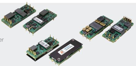
Advanced Energy's Artesyn ADO300 series eighth-brick isolated DC-DC converters provides a single fully regulated at 3.3V, 5V or 12 V output. Rated at 300 watts, these converters can deliver up to 300W power and have no minimum load requirement. They have an input voltage range of 36 to 75 V and are primarily designed for use with standard 48 V supplies in computing and server applications, as well as regulated 48V supplies in communications equipment.
