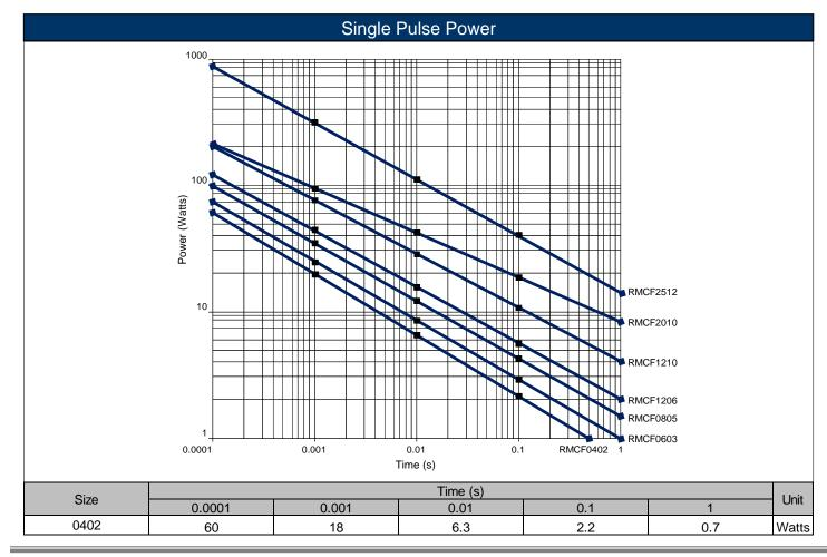
General Purpose Thick Film Standard Power and High-Power Chip Resistor
