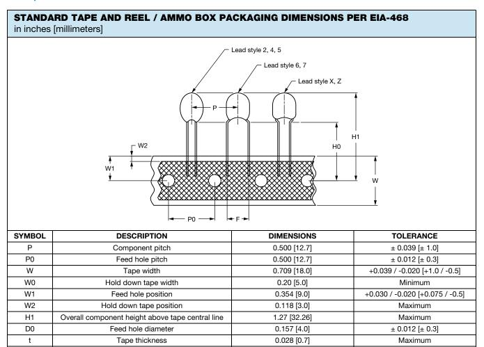
**Tape and Reel Packaging:** type 199D radial-leaded tantalum capacitors, all lead styles except 1, 3, and Y are available taped and reeled per EIA-468.
