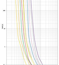
30 A - 150 A: FI = 1.25 (max. operating current:0.8 x I<sub>rat</sub> at 23°C) 200 A: FI = 2.00 (max.operating current: 0.5 x I<sub>rat</sub> at 23°C)
