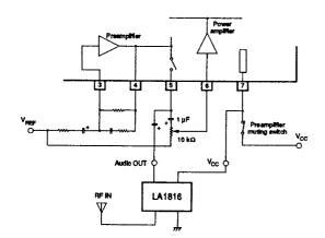
The internal circuit of the POWER MUTE pin is shown in the following figure.
