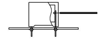
Temperature monitored inside the capacitor.
