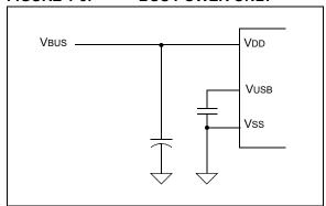
In order to meet the inrush current requirements of the USB 2.0 specifications, the total effective capacitance appearing across VBUS and ground must be no more than 10  $\mu$ F. If it is more than 10  $\mu$ F, some kind of inrush limiting is required. For more details on inrush current limiting, search for that subject in the latest "Universal Serial Bus Specification".
