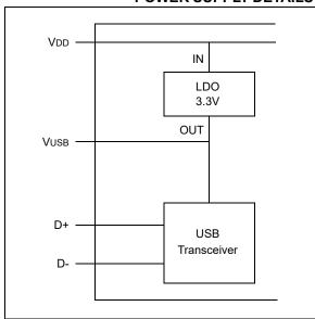
The provided VDD voltage has a direct influence on the voltage levels present on the GPIO and UART Tx/Rx pins. When VDD is 5V, all of these pins will have a logical '1' around 5V with the variations specified in Section 4.1 "DC Characteristics".
