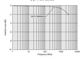
■ Differential Mode Transmission Characteristics (Typ.)
