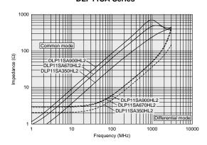
■ Differential Mode Transmission Characteristics (Typ.)
