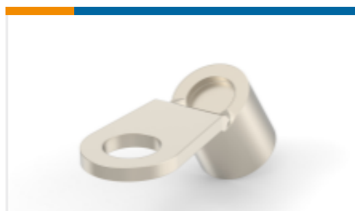
TE Part #1958523-4 STRATO, R, HR, 6, M6(1/4), NIPL, 60 BEND
