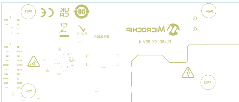
Figure 5-12. PL460-EK Layout: Bottom Silkscreen
