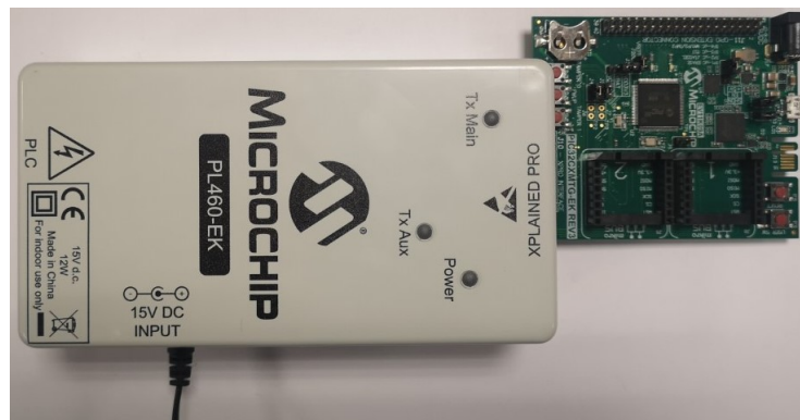
Figure 2-2. Connection of AC/DC Wall Adapter and Host
