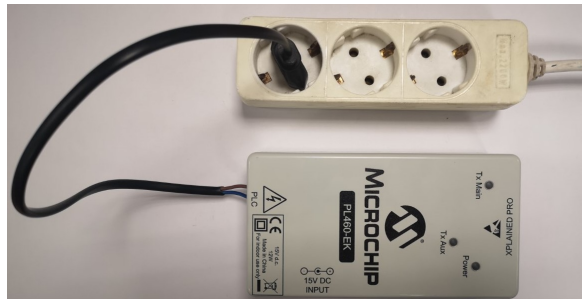
Figure 2-7. PL460-EK Powered from Mains Grid with Closed Enclosure
