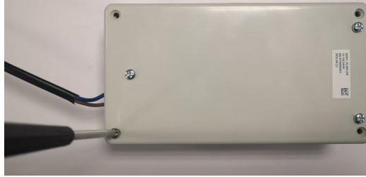
Figure 2-6. Screws of the Lid to Close the Enclosure
