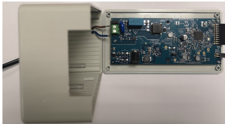
Figure 2-4. Cables through the Holes of the Enclosure
