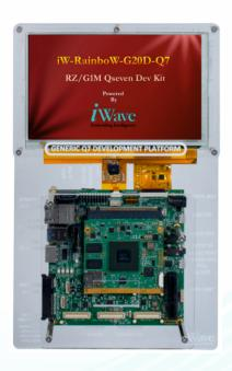
iWave's RZ/G1M,G1N development board incorporates RZ/G1M,G1N QSeven SOM which is based on Renesas high performance RZ/G1M,G1N Dual ARM Cortex A15 MPU and the carrier board with optional 7" capacitive Display Kit. The development board can be used for quick prototyping of various applications targeted by the RZ/G1M,G1N processor. With the 120mm x 120mm Nano ITX size, the kit is highly packed with all the necessary on-board connectors to validate the RZ/G1M,G1N MPU features.
