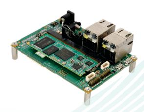
iWave's i.MX6ULL development board incorporates i.MX6ULL SODIMM SOM which is based on NXPs power efficient i.MX6ULL ARM Cortex A7 processor and the carrier board with optional 4.3" resistive display kit. The development board can be used for quick prototyping of various applications targeted by the i.MX6ULL processor. With the 100mm x 72mm Pico ITX size, and the kit is highly packed with all the necessary on-board connectors to validate the i.MX6ULL CPU features.
