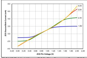
**FIGURE 35-117:** ZCD Pin Current Over ZCD Pin Voltage, Typical Measured Values From -40°C to 125°C.
