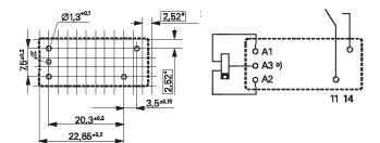
PCB layout / terminal assignment
