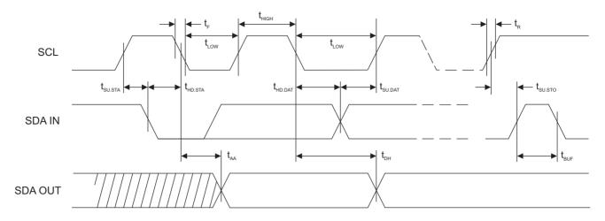
Figure 6-6. Write Cycle Timing
