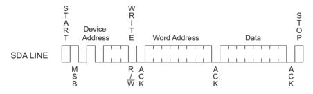
**Page Write:** The 1-Kbit and 2-Kbit EEPROM are capable of an 8-byte Page Write.
