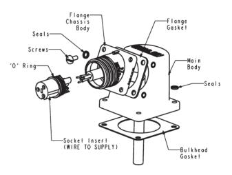
Fig 4. Flange/Bulkhead Mounting (PX0941 + PX0950)
