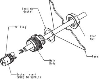
Fig 3. Chassis/Panel Mounting (PX0931)
