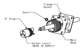
Fig 5. Flange Mounting (PX0941)
