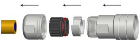
Step 1: Slide parts onto cable
