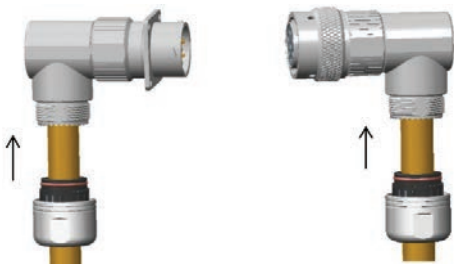
Step 11: Push shielding clip into backshell
