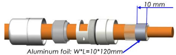
Step 4: Wrap foil over braided shielding
