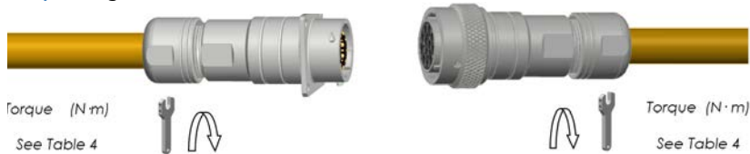
Step 13: Tighten metal nut
