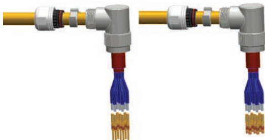
Step 7: Attach contacts to wire leads
