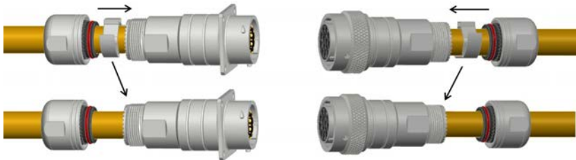
Step 11: Push shielding clip into backshell
