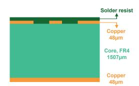
Figure 14. PCB stack-up recommendations
