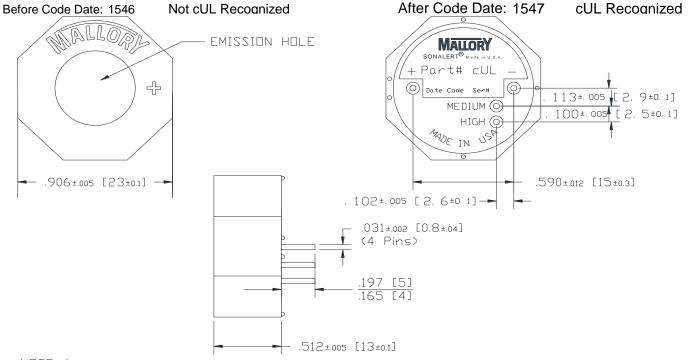
NOTE A: TERMINALS - .031" DIA. NICKEL/TIN COATED BRASS. NOTE B:
