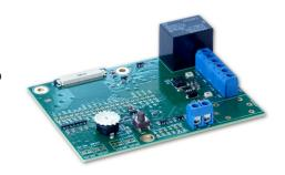
Power supply is 5~30V= at screw terminal J5. We suggest to provide around 12V= if provided fan is used. An onboard voltage regulator generates 3.3V (VDD) for display and relay.
