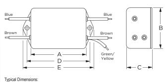
Wire Leads (5): Mounting Holes (2): 4.0 [101.6] Min., AWG18 .188 [4.78] Dia.
